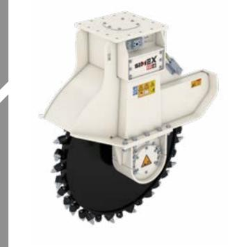
For excavator boom mounting, RWE 60 wheel saws are designed to make set-section cuts on hard and compact surfaces: asphalt, concrete, rock.
